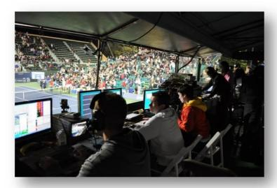
During ITF testing in 2006 Hawk-Eye passed a number of stringent parameters, meaning that it would be the first electronic line calling system to be officially accredited. Results showed the system to have a mean error of only 2.6mm when compared to a high speed camera located on the playing surface.
